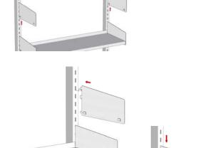
f. Align the upstand shelf with the endplate shelf lugs and lower into position.
