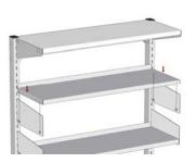
g. Ensure that the shelf fits securely and level in the lugs by firmly pressing towards the base of the post. Note! The shelf should be fully seated in the lugs as shown.
